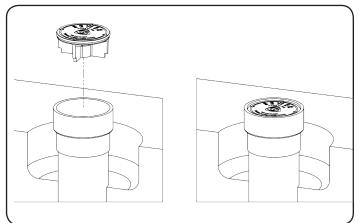
Install the Sewer Seal Cap into the fitting and press down until the cap is fully seated into the fitting. When properly install the cap will be slightly below the fitting.
