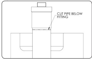
Mark the pipe just below the fitting. Cut the pipe and remove the existing fitting.
