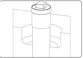
Excavate the access pipe to expose at least 4" of pipe. The hole should be large enough to cut the pipe.
