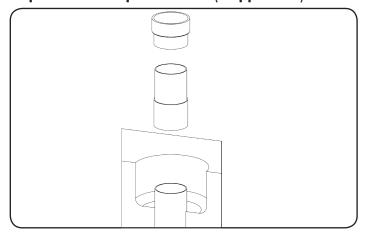
If the pipe is too short after removing the old fitting leaving the new cap below grade or below the desired height, an extension pipe will need to be added. Using a coupler and a short piece of pipe, raise the cleanout to the desired height. Then cement the fitting as described in step 4.
