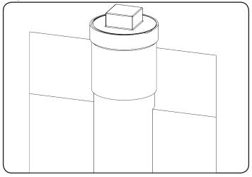
These instructions detail how to replace a standard threaded PVC access cover with the Argonics Sewer Seal.
