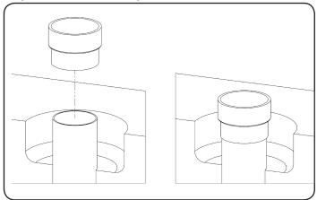
Clean the outside of the pipe with PVC Cleaner. Also clean the inside of the new adapter or coupler. Cement the new fitting to the pipe.
