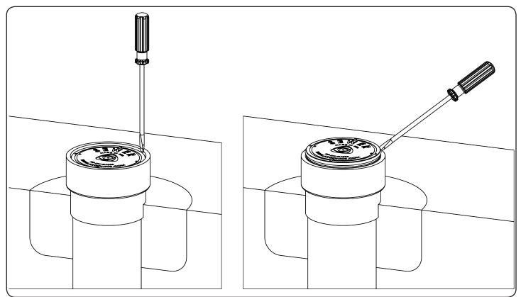
To remove the cap insert a screwdriver between the PVC fitting and the cap. Push the screwdriver down past the seal on the cap, approximately  $\frac{1}{2}$ ". Then gently pry the cap up. The cap will pop up and it can be removed by hand.
