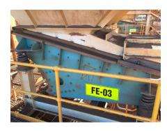
To control the feed to their screen, the conveyed material is put through a Schenk Vibratory Feeder. However, due to the level of product build-up occurring on the existing Bisalloy plate chute lining (.78" (20mm) hardox 450), the customer had to stop the plant 3-4 times per shift to jack hammer the iron ore manually.
