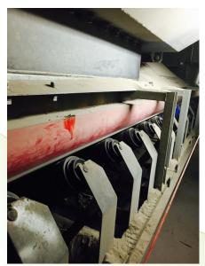
During production stoppages, manual resources were required on a frequent basis to shovel clear the area around the chute system. Not only did this create a physical abor **OHS issue**, but breathing in the airborne particles runs the risk of leading to more grave health issues.
