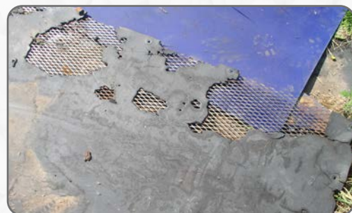
These are a competitor's ester-based sheets, which have failed in a humid environment. This deterioration is called hydrolytic degradation.
