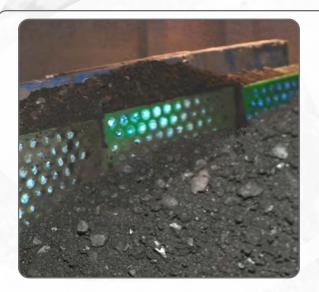
Redi-Liner bolt-in 12"x12" panels can be arranged into any wear pattern that is needed. Their unique, simple installation method allows you to replace only what's needed instead of replacing the entire liner.
