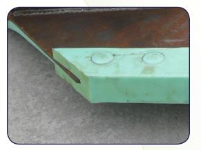
The blade liners are made from the same material as the Evolution liner, so they have the same wear properties and use the same Snap-Tite plugs.
