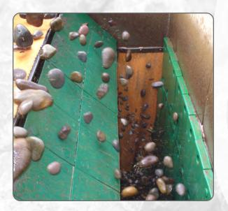
Wear plates help eliminate material adhesion and dampen noise levels significantly. Our polyure-thane wear plates have proven to be cost-effective over steel liners by as much as 5-to-1.
