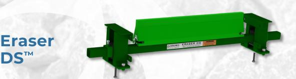
The Eraser DS is an economical version of our XTC cleaner, with a .19" thick, 2"x 2" powder-coated tube stock steel mainframe for strength and durability. The DS uses the same polyurethane blade as the XTC.
