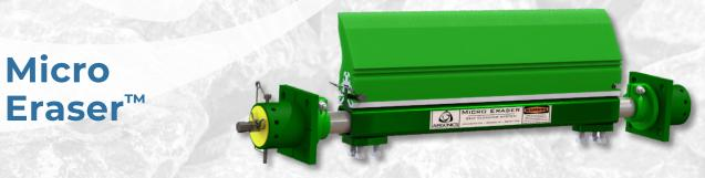
The Micro Eraser is your answer for portable equipment with tight clearance issues. Designed with our 6" tall polyurethane blade, it works best on belts up to 48" wide with head pulleys of 28" diameter or less. This economical but powerful system uses our patented Perma-Torque™ tensioner.
