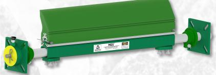
The MES cleaner is a low-maintenance, high-performance cleaner with a low-profile, compact design. It uses our 6" tall polyurethane blade, and the universal mounting plates are designed to allow the cleaner to replace other OEM conveyor cleaners. The MES uses a unique internal tensioning system that allows for quick and easy tensioning.
