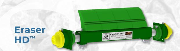
The Eraser HD is designed to withstand heavy vibration. This system has a reinforced mainframe and a heavy-duty channel attachment design. It utilizes a series of 6'' wide x 7'' tall polyurethane blade segments that conform to crowned head pulleys.
