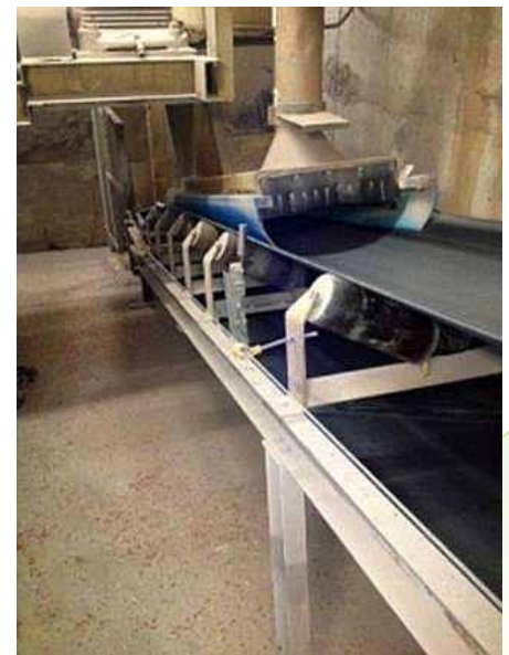
Photos of Snap-Loc installed around the transfer point. The blue polyurethane indicates the Flame Resistant, Anti-Static (FRAS) properties.
