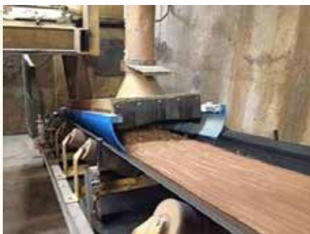
Photos of Snap-Loc installed around the transfer point. The blue polyurethane indicates the Flame Resistant, Anti-Static (FRAS) properties.
