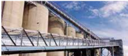
Photos of Snap-Loc installed around the transfer point. The blue polyurethane indicates the Flame Resistant, Anti-Static (FRAS) properties.
