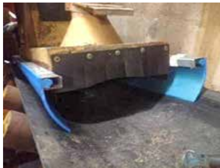
Photos of Snap-Loc installed around the transfer point. The blue polyurethane indicates the Flame Resistant, Anti-Static (FRAS) properties.
