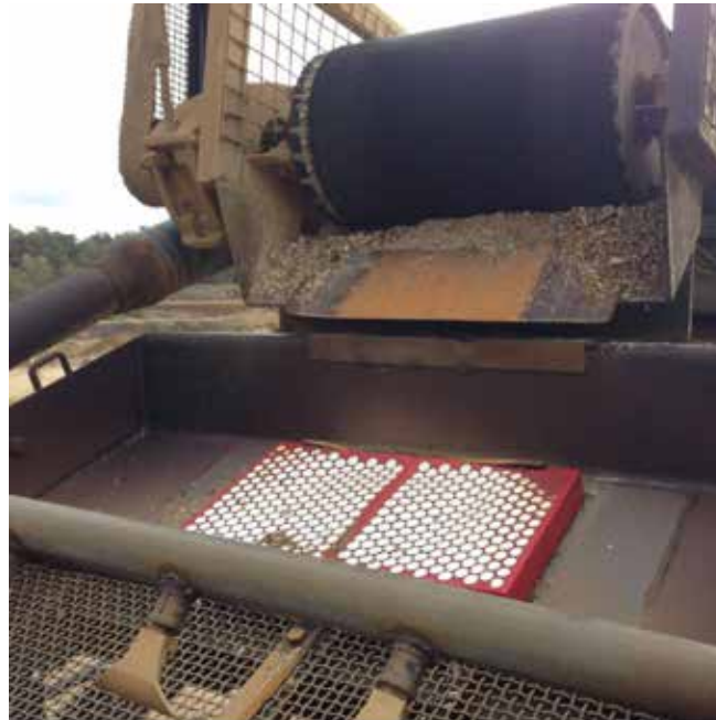
2013 photo of Redi-Liner ceramic lining still in place after 2 years and 4 months of constant use
