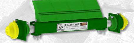
The Eraser HD is designed to withstand heavy vibration. This system has a reinforced mainframe and a heavy-duty channel attachment design. It utilizes a series of 6'' wide x 7'' tall polyurethane blade segments that conform to crowned head pulleys.
