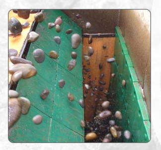
Wear plates help eliminate material adhesion and dampen noise levels significantly. Our polyure-thane wear plates have proven to be cost-effective over steel liners by as much as 5-to-1.
