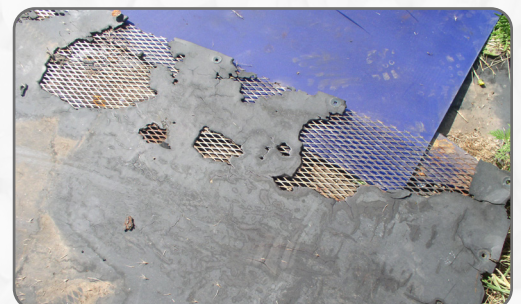
These are a competitor's ester-based sheets, which have failed in a humid environment. This deterioration is called hydrolytic degradation.
